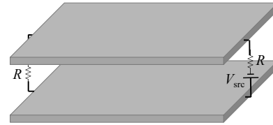
Fig. 13: Geometry and excitation used for the parallel plate capacitor in Section VI-F.
