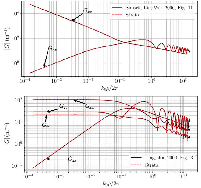
Fig. 1. Accuracy validation for Strata. Top: Comparison to Fig. 11 in [7]. Bottom: Comparison to Fig. 3 in [12].
